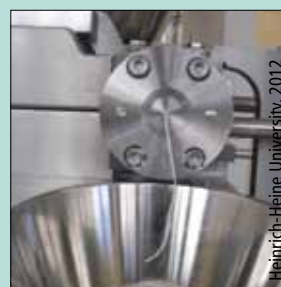
Lactose / MCC 80:20, 1mm die, Powder feeding rate 2g/min, liquid feeding rate 1.07g/min
