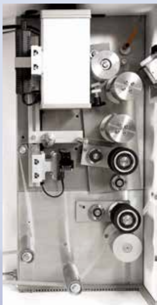
Film take-off part with Film Quality Analyzer
