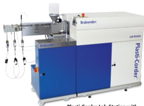
Plasti-Corder Lab-Station with measuring extruder 19/25
