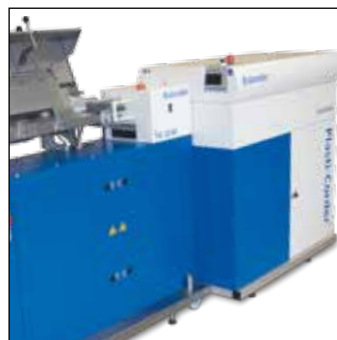
Plasti-Corder Lab-Station with twin screw extruder TSE 20/40
