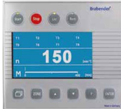
Control panel for parameter setting and display of the measured values
